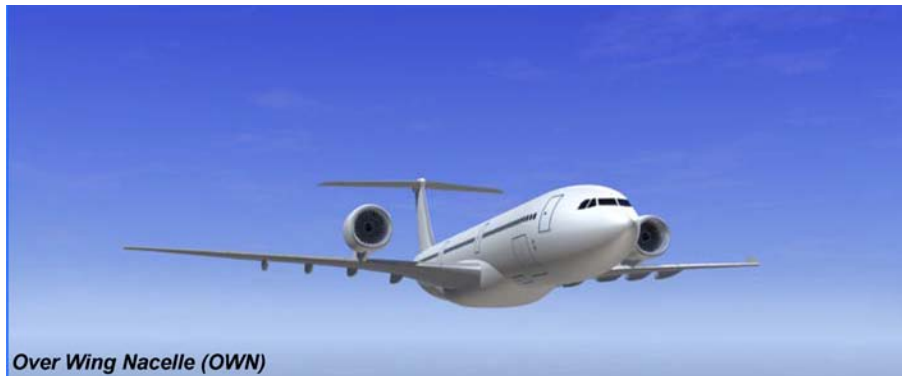
Figure 105: Configurazione Over the Wing Nacelle .
