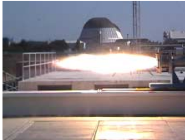
Figure 11.10 Hybrid motor test at NASA Ames. Thrust is approximately 2500 pounds with a simple convergent nozzle.
